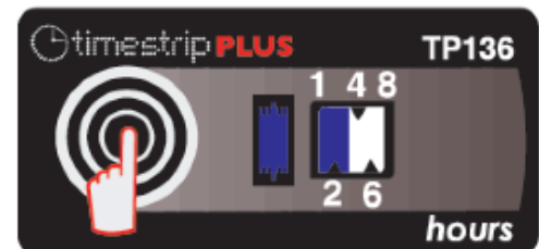
Activated Threshold temperature exceeded for more than 2 hours.
